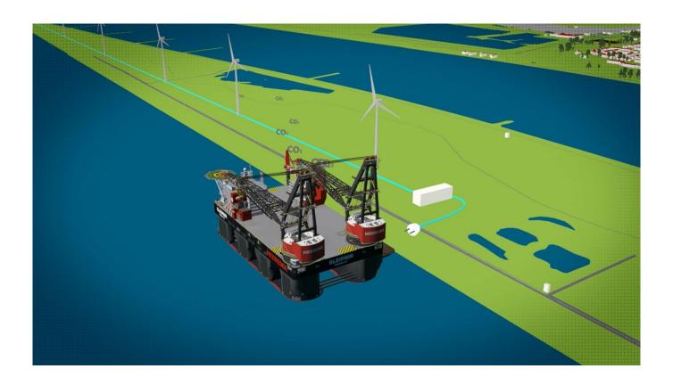
Heerema's Shore Power Caland Canal project will revolutionize how we power our vessels when they are in port. When moored in Rotterdam, Heerema's vessels will be connected to the wind turbines on the Rozenburg headland, ensuring noise, and emissions that can be associated with moored vessels will be replaced by green, quiet, emission-free energy.
